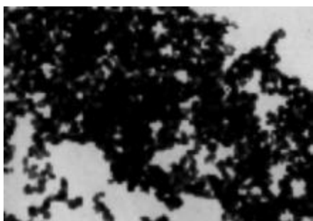
图4 HF 提取物与硅酸反应形成的颗粒状硅沉淀(×1 000) Fig.4 Particles of silica precipitation from reaction of HF extract and silicic acid (×1 000)
